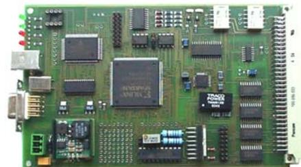
**Figura 2.** Tarjeta IAEA DAQ-52.
