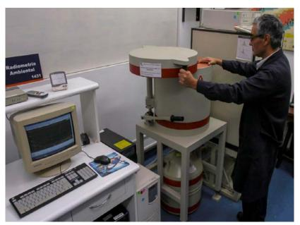
Figure 3. Gamma spectrometry system.
