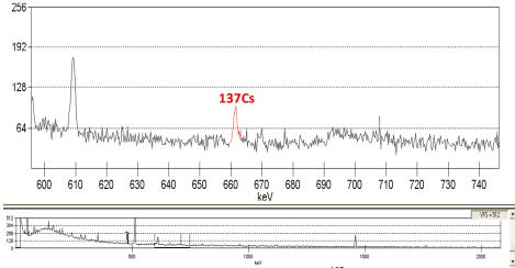
**Figure 4.** Gamma spectrum of <sup>137</sup>Cs.
