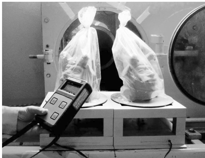
Figure 2. The irradiation facility, loaded with two replicates.
