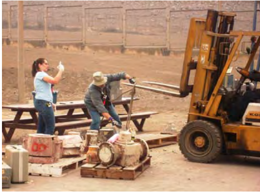
Figure 4. Removal of disused sealed sources.
